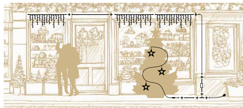
EXAMPLE OF MIXED 230V AND 24V WIRING
